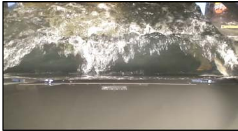
Figure 11. Top-view of periodic wave breaking showing typical triangular structure.
